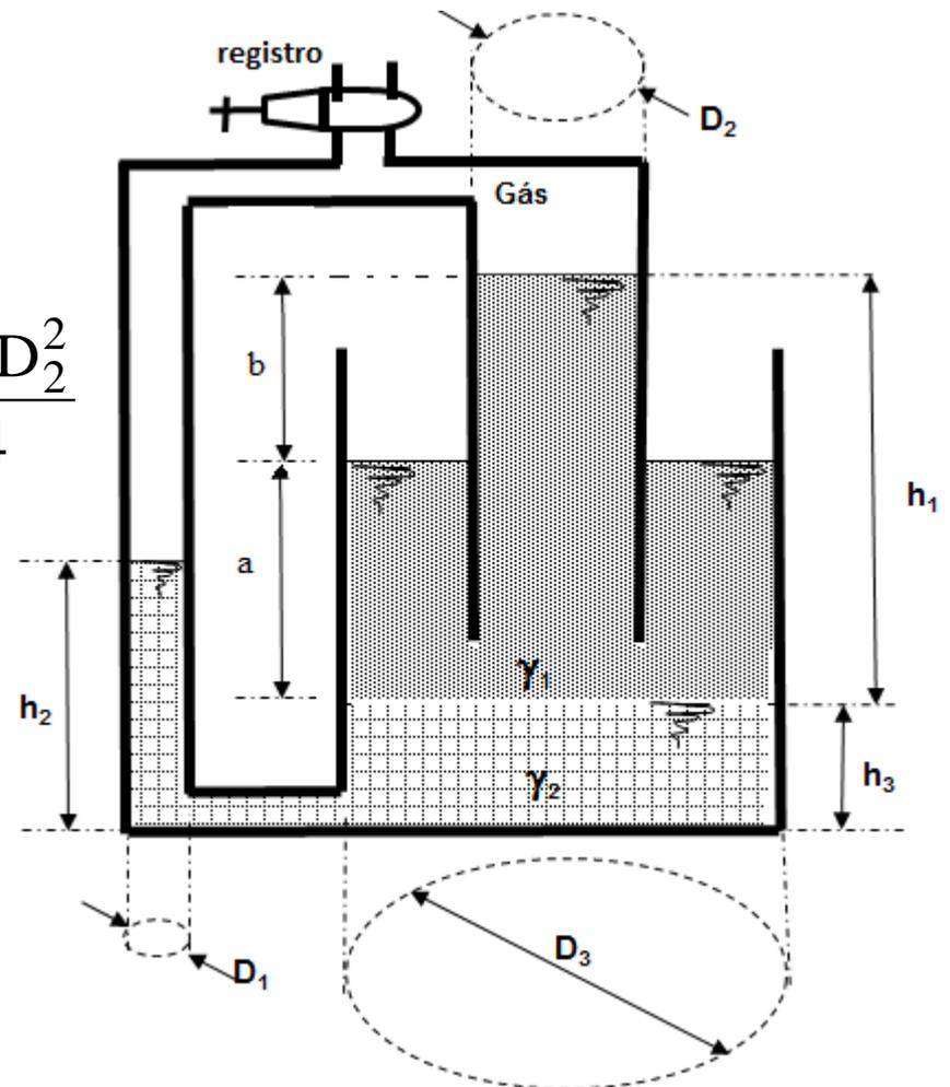
$$a \times \frac{\pi \times D_3^2}{4} + b \times \frac{\pi \times D_2^2}{4} = h_1' \times \frac{\pi \times D_3^2}{4}$$
