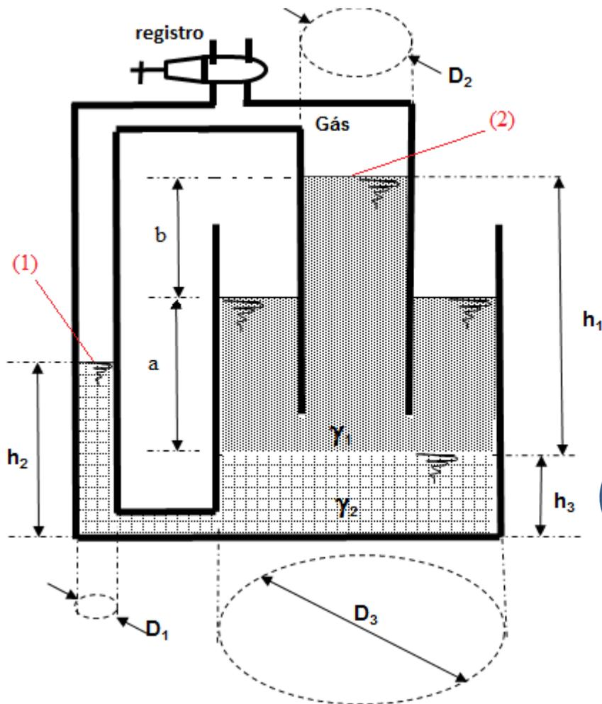
$$p_{\text{gás}} + \gamma_2 \times (h_2 - h_3) - \gamma_1 \times h_1 = p_{\text{gás}}$$
