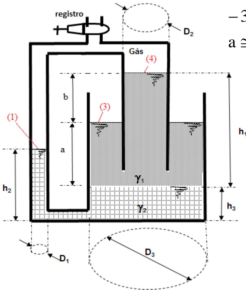
$$p_{\text{gás}} + \gamma_2 \times (h_2 - h_1) - \gamma_1 \times a = 0$$
