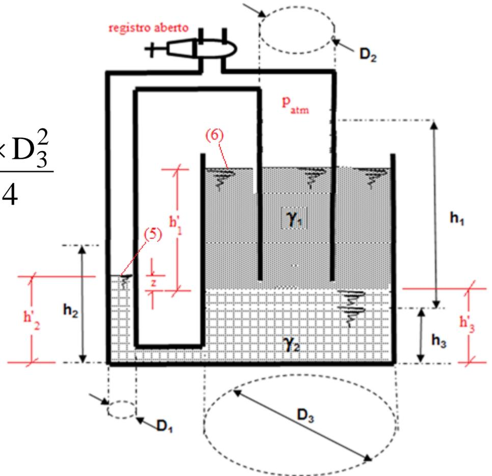
$$a \times \frac{\pi \times D_3^2}{4} + b \times \frac{\pi \times D_2^2}{4} = h_1' \times \frac{\pi \times D_3^2}{4}$$
