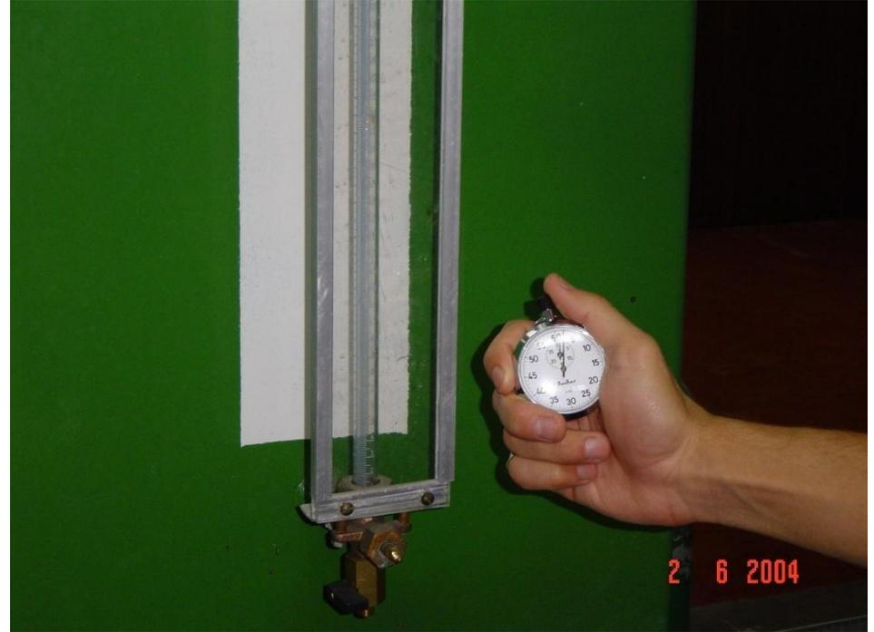
$$Q = \frac{\text{Volume}}{t} = \frac{A_{\text{tanque}} \times \Delta h}{t}$$
