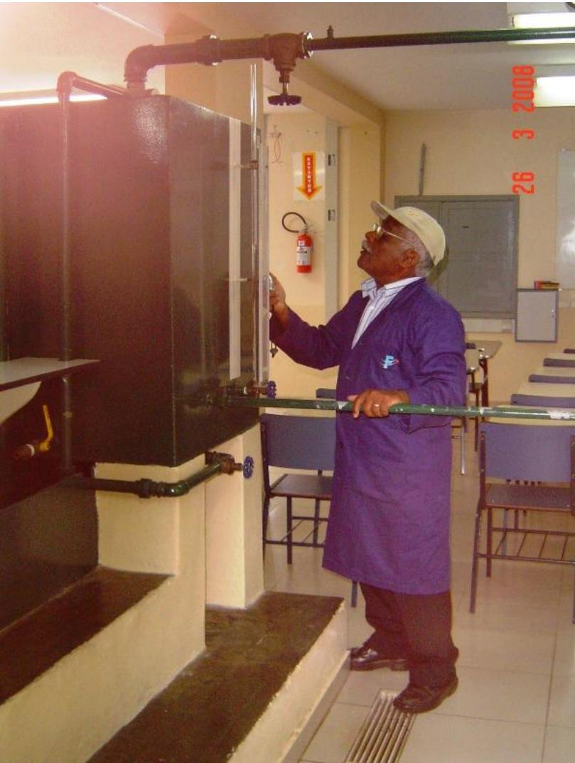
$$Q = \frac{\text{volume}}{\text{tempo}} = \frac{\Delta h \times A_{\text{tanque}}}{t}$$
