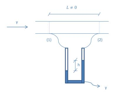
$$\begin{split} H_1 &= H_2 + h_{f_{1-2}} \\ h_{f_{1-2}} &= \frac{p_1 - p_2}{\gamma} = h \times \left(\frac{\gamma_m - \gamma}{\gamma}\right) \\ Q &= \frac{\Delta h \times A_{tan \, que}}{t} \rightarrow v = \frac{Q}{A} \\ f &= \frac{h_{f_{1-2}} \times D_H \times 2g}{L \times v^2} \end{split}$$
